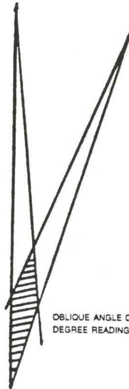
OBLIQUE ANGLE CROSSED BEARINGS, FIVE DEGREE READING ERROR
